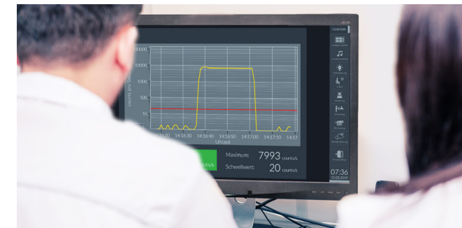
EXT-RAD-0002 Radiation Detection Whether as an additional safety instance in teletherapy or as an operational requirement in brachytherapy, the residual radiation in the room is reliably measured independently of the source, the values are digitally documented and, if the threshold values are exceeded, a warning is given before the radiation protection door is opened.
